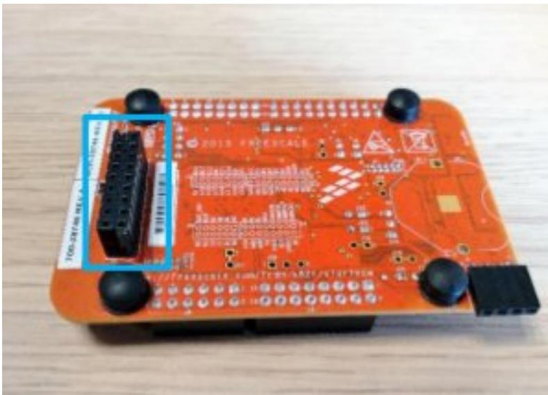
2. Install OpenSDA for the NXP K82F board More information can be found at [segger website](#). Click on **J-Link OpenSDA - Board-Specific Firmwares** and download the firmware for the **FRDM-K82F**.
