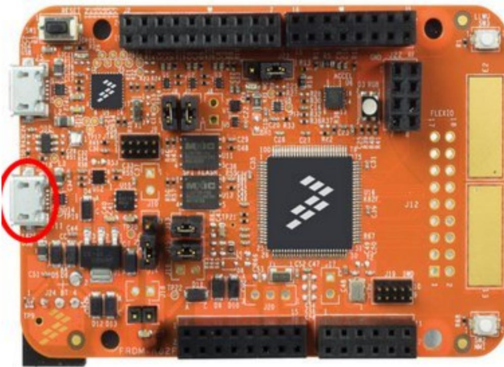
3. The board will enumerate as a generic USB video device called **Flexio Camera Device**. You can then use this device with any video capture software such as “camera” from Windows 10 or *AMCap*. Download and install it if you don’t have camera application on your O.S. Launch it and select the **Flexio Camera Device** device. You will see the frames transmitted at a resolution **QQVGA** of **160x120** pixels.
