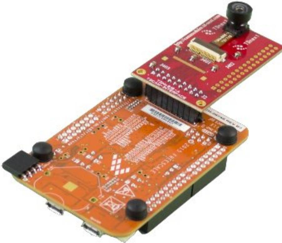
6. Plug in the **micro USB** cable in the USB device port (the one in the middle of the card).
