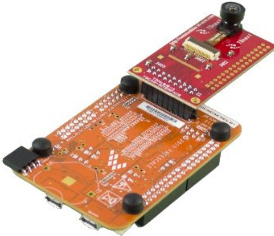
*FRDM-K82F with TDNx016 board mounting a TD7740 camera module*
