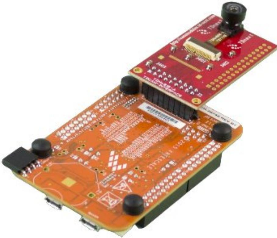
2. Plug in the **micro USB** cable in the USB device port (the one in the middle of the card).
